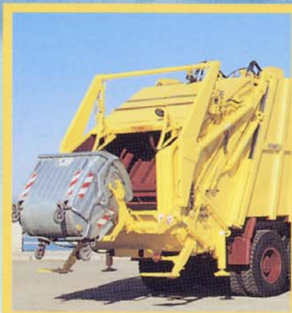
Dispositivo voltacassonetti / Bin-lifting device / Lève-conteneurs.
